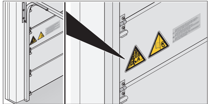
Fig. 1.2 Attach sticker on door panel
