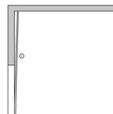
VLU: Vertical lift fitting with underlying torsion spring shaft
