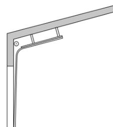
HLD: High lift guide rail fitting following roof line (max. 30°)
