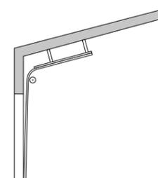
HLDU: High lift guide rail fitting following roof line and underlying torsion spring shaft
