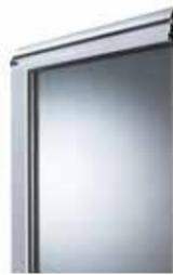
Frame profile with 20 mm synthetic double glazing, tinted green; light transmission of approx. 70%
