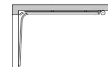
NSH: Low-headroom fitting with rear-mounted spring shaft
