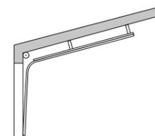
ND: Normal fitting following roof line (max. 30°)
