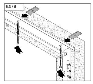
• Drill through all the pre-marked holes of the side frame into the wall.
