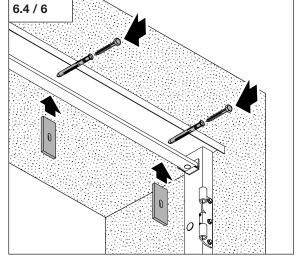
• Drill through the elongated holes of the fastening brackets.
