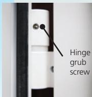
The polymer hinge bearing can be aligned in one of four positions - remove the door leaf, unseat the bearing and rotate to the desired position (see right). The hinge pin can also be adjusted - see below.
