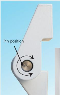
The hinge pin and polymer hinge bearing are both acentric and allow for +/- 0.75mm adjustment each to the hinge position. The dot on the top of the pin shows its position and this can be adjusted with an allen key inserted into the bottom of the pin (release the grub screw in the hinge to allow adjustment).
