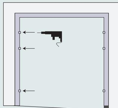
**When drilling ensure all parts of the door are protected from brick dust and other fragments.**
