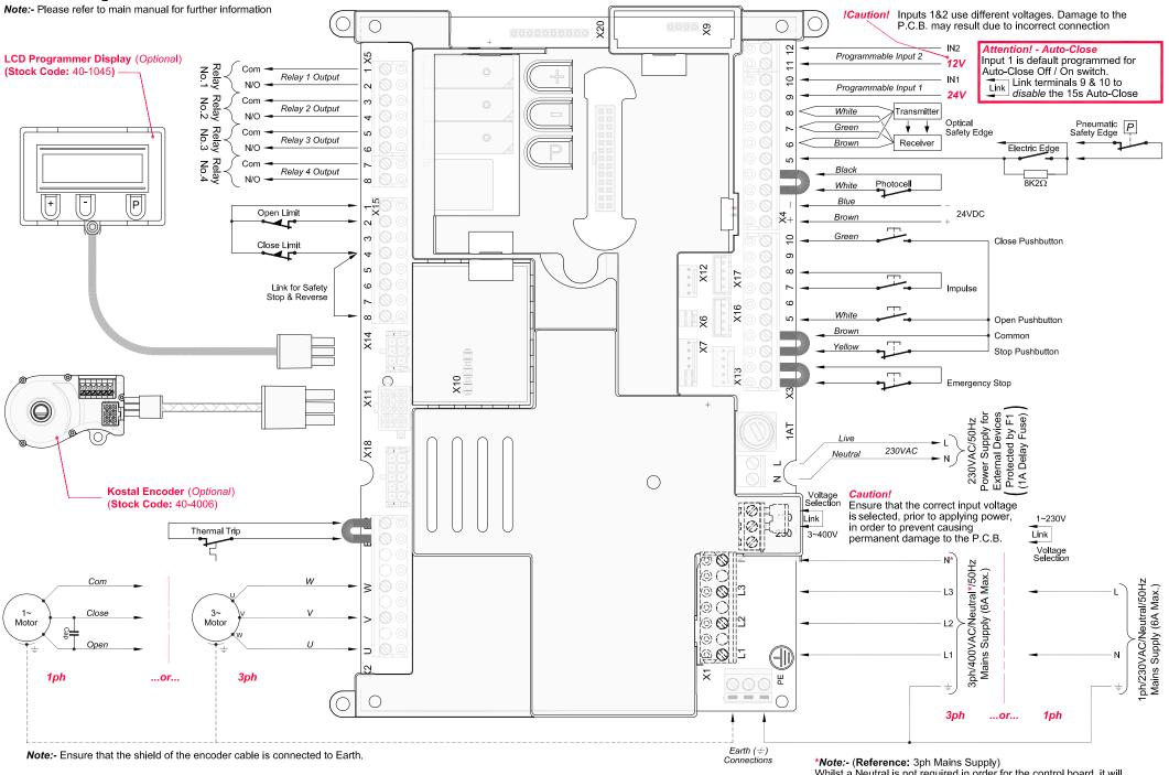
Whilst a Neutral is not required in order for the control board, it will prevent the use of the auxiliary 230VAC supply provided on X19
