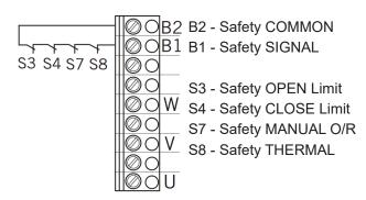
The limit system will be recognised automatically by the control during initial use. If replaced at a later date, the relevant limit system must be selected in a parameter setting in the INPUT operating mode.
