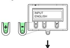
Press the '+' button to scroll through the menu until 'INPUT 1' is reached
