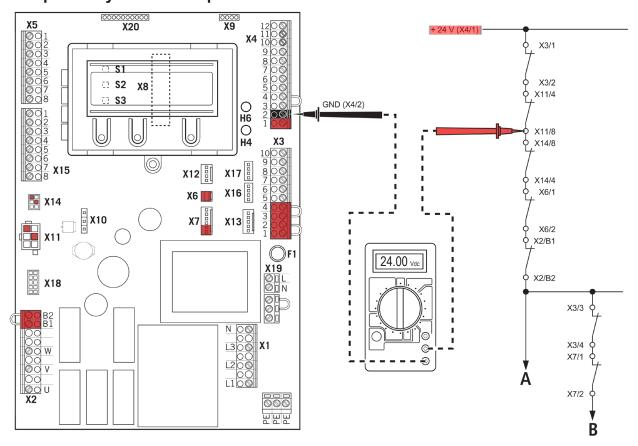
The multimeter must be set for 24 Vdc. Measure at all test points on the diagram to locate the fault.
