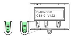
Press and hold the 'P' button until 'AUTOMATIC' is reached Programming is now completed
