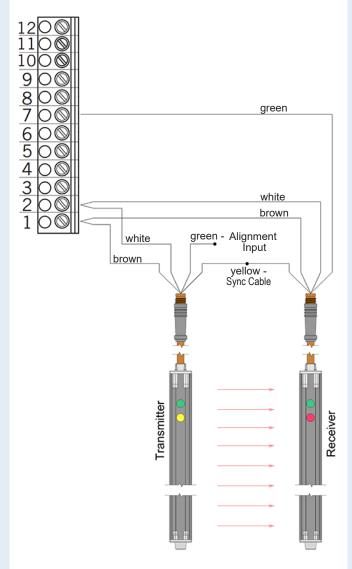
Safety edge mode 'SKS' should be set to MOD4 for light curtain operation (not automatically detected).
