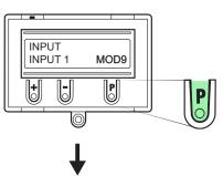
Press both '+' and '-' buttons together to exit the 'INPUT' menu
