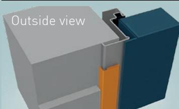
The FB Frame option allows for a flush finish between door lip, frame and wall finish on Corner and Corner Counter frames in new openings that are rendered after the door is installed. The FB option also provides a flush finish on block frames that are fixed at the front edge of the garage opening reveal.
