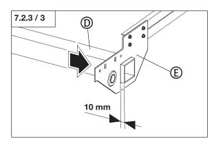
• Secure the hollow profile (D) at both sides of the side console with bearings (E).
