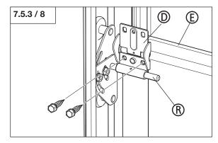
• Screw all the required central hinges (G) onto the door section.
