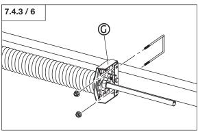
• Push the shaft coupling (H) onto the spring shaft (C).
