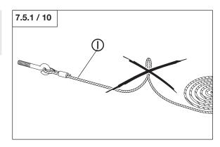
The cables may be longer than required upon delivery. To facilitate cable installation, mark the correct length on the cables in advance.
