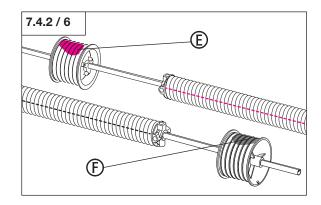
• Insert the spring shaft (G) into the bearing console.
