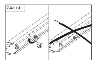
• Screw the triangular console to the lateral rail.
