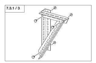
• Screw the clamping bolt (B) into the C-shaped profile of the lateral rail with the correct orientation.
