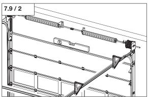
If the door leaf is not in a horizontal position, it can be adjusted via the eyebolt (A) at the bottom console. The eyebolt is adjusted via the respective nut (B).
