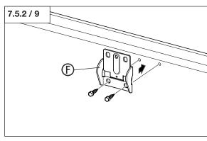
• Assemble all the other door sections, side hinges, rollers and central hinges.
