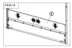
• Insert the spacers between the sections
