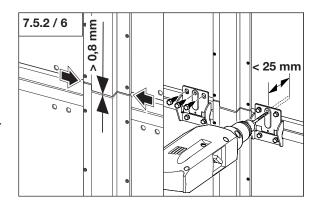
• Screw all the hinges of the bottom section to the other door section.
