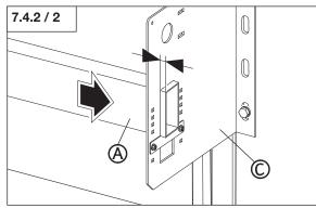
• Secure the hollow profile (A) on both sides to the side consoles with bearings (C).
