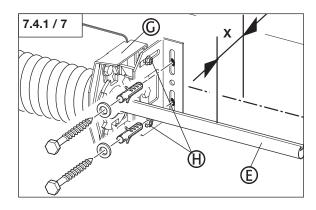
• Push the shaft coupling (I) onto the spring shaft (E).
