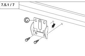
• All side and central hinges must be lubricated after installation.
