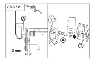
• Screw the tandem roller with guide cylinder (A) to the floor section.
