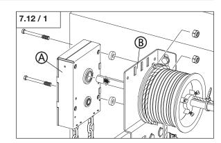
• Screw the geared chain retainer (C) to the frame.
