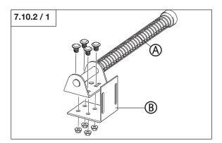
• Screw the bracket (B) hand-tight to the lateral guide rail.
