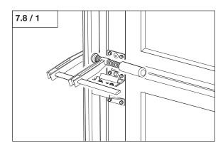
The correct spring tension depends on the size and weight of the door.
