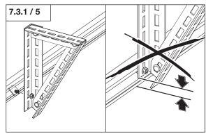
• Screw the suspension to the roof.
