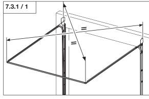
The number of required suspensions (A) depends on the length (X) of the lateral rails.
