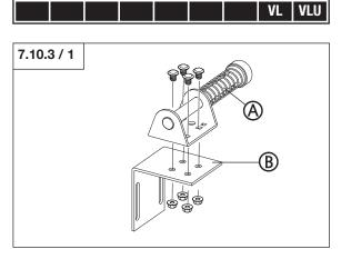
• Screw the bracket (B) to the upper end of the lateral rail (C).
