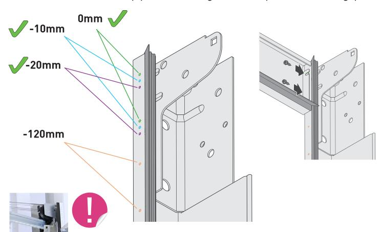
**-120mm** sits 120mm down from the top of the frame leg. Use this position when fitting a 240mm headroom kit - it drops
