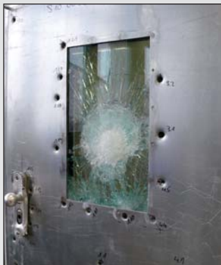
Exhaustive testing of the door leaf and glazing confirmed that the design meets the resistance requirements of Class FB 4.
